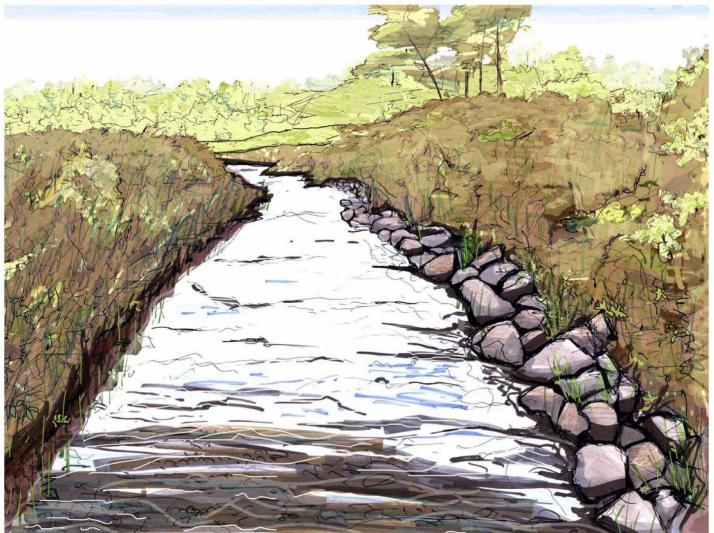
Stone Toe Protection is constructed from cobble-sized rock on the creek edges. It extends to approximately the bankfull level, which will protect the channel banks for flow events that occur every 1 to 2 years or less. The material will extend into the ground to resist scour. Coarse gravel is used to separate the larger rock material from underlying soil. Stone toe protection is typically used in conjunction with revegetation of the upper
