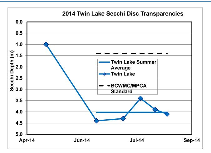
Figure 38 2014 Twin Lake Secchi Disc Depths Compared with BCWMC/MPCA Secchi Disc Standard
