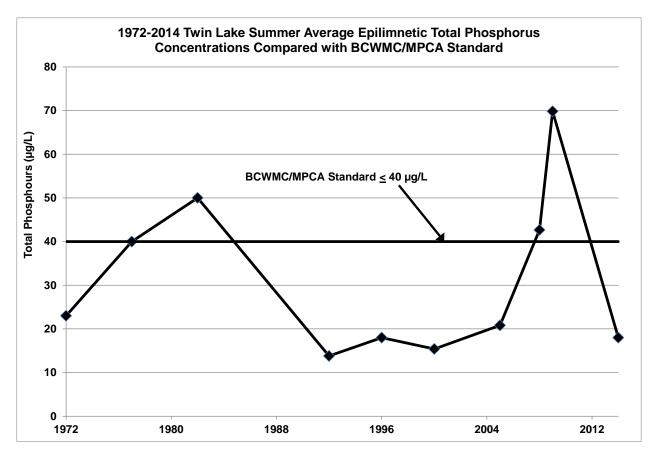
Figure 49 1972–2014 Twin Lake Total Phosphorus Concentrations Compared with BCWMC/MPCA Total Phosphorus Standard
