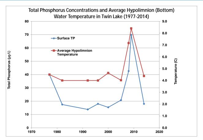
Figure 52 Total Phosphorus (TP) Concentrations and Average Bottom Water Temperatures in Twin Lake (1992–2014)
