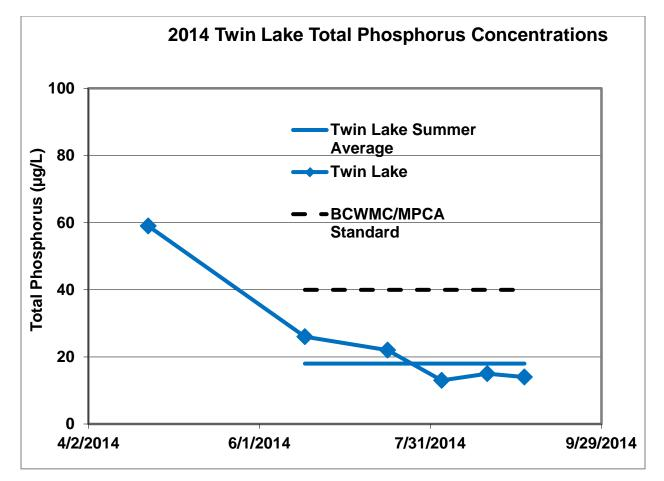
Figure 36 2014 Twin Lake Total Phosphorus Concentrations Compared with BCWMC/MPCA Total Phosphorus Standard
