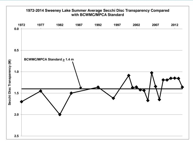
Sweeney Lake Historical Secchi Disc Depths Compared with BCWMC/MPCA Figure 27 Secchi Disc Standard
