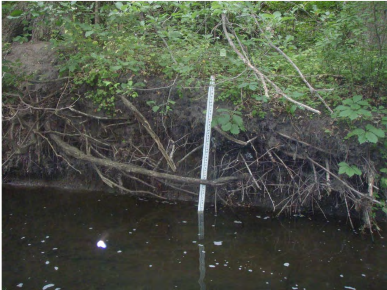
Photo 20. Site 18. Moderate erosion with undercut trees.
