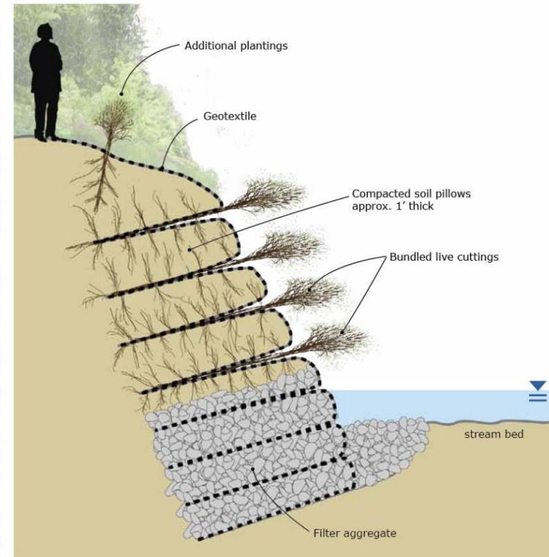
In places where the channel is confined by the steep valley walls, however, fluvial bank erosion can lead to failure of the high banks. It can also undermine storm sewer inlets. For sites where groundwater seepage is a problem and where it is desirable to maintain steep banks, soil pillows are a feasible solution.
