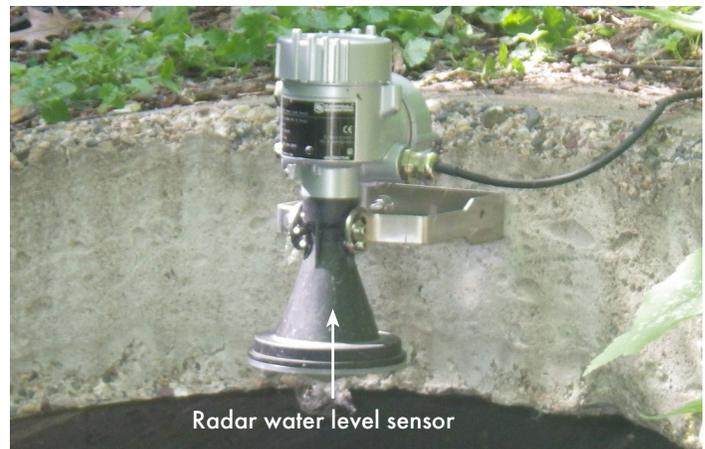
Figure 2: Radar water level sensor
