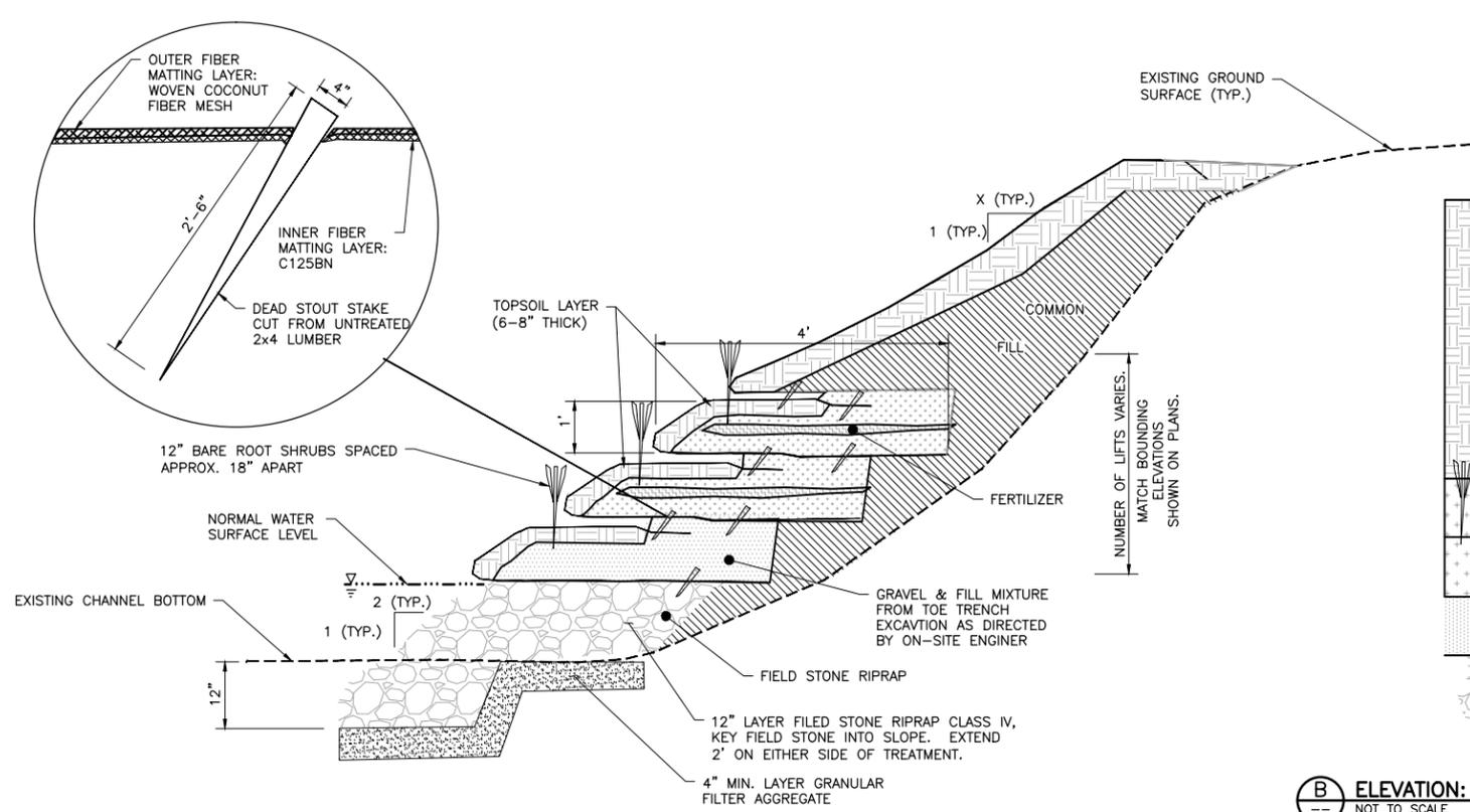
**A SECTION: LIVE PLANT VEGETATED REINFORCED SOIL SLOPE (V.R.S.S.)**
