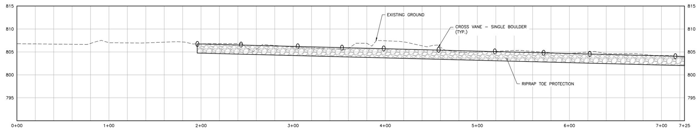
**2 PROFILE: REACH 4 (STA. 0+00 TO 7+00)** 0 30 60 HORIZONTAL SCALE IN FEET 0 6 12 VERTICAL SCALE IN FEET
