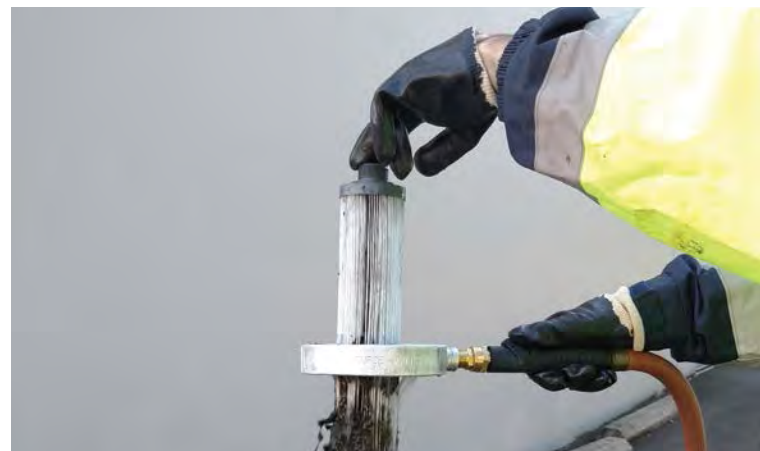
The Jellyfish® Filter tentacle is light and easy to clean.
