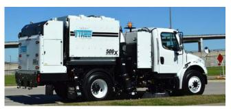
lakes. This new sweeper uses a different mechanism than older sweepers and is more effective at collecting fine material. In addition to targeting high priority areas around waterbodies, it will sometimes be operated behind the mechanical broom sweeper in the spring and fall and will be used during the city's mill and overlay projects to collect debris before it's washed into storm sewers.
