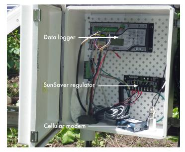
Figure 3: Data logger, cellular modem, and SunSaver regulator
