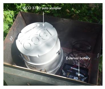
Figure 5: Automatic sampler and external battery
