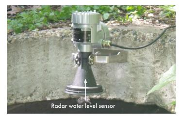
Figure 2: Radar water level sensor
