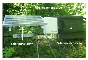
Figure 4: Solar panel, flow logger enclosure, and auto sampler shelter
