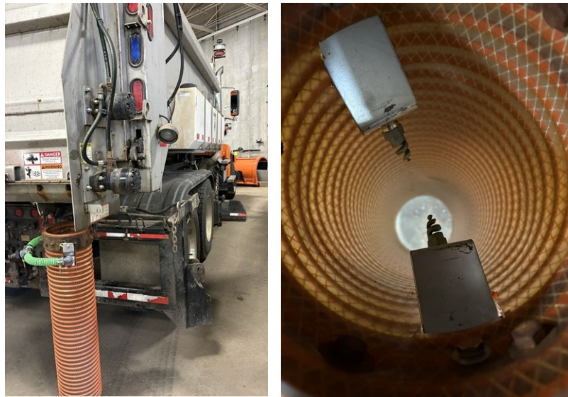
Plymouth truck station agriculture pipe with fan sprayers for prewetting
